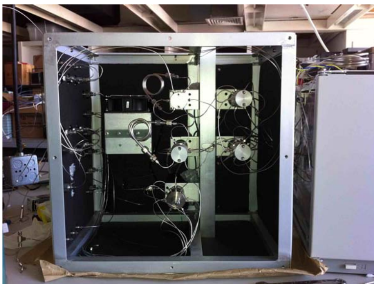
Figure 2-2: The sample module containing valves, sample loops, Nafion dryer and inlet ports is held at 35°C to correct for any variations in sample amount between the air sample and standard.
