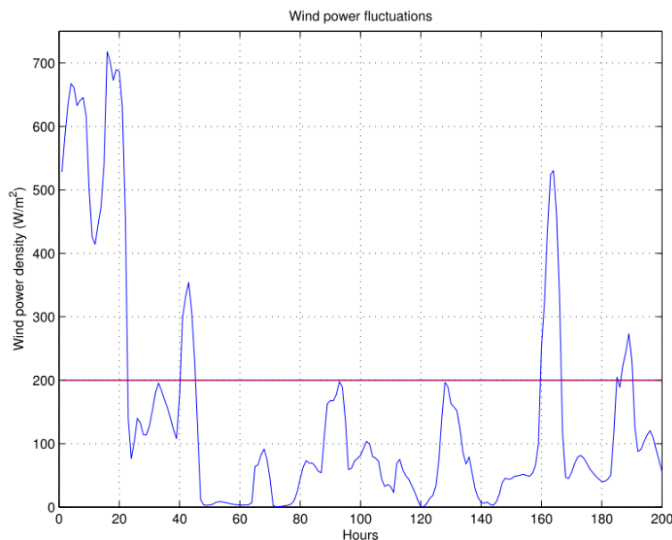
Figure 18. Illustrative wind power density profile showing fluctuations in wind, from Gunturu and Schlosser (2011).
