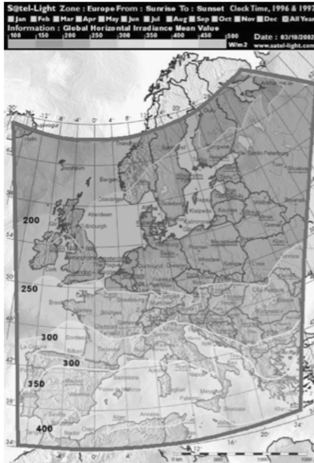
Figure 4. Geographical variation of the annual mean shortwave flux based on the years 1996 and 1997, averaged over the sunshine duration. Units are in W/m 2 . (Source: Hammer et al. (2003), Figure 5).
